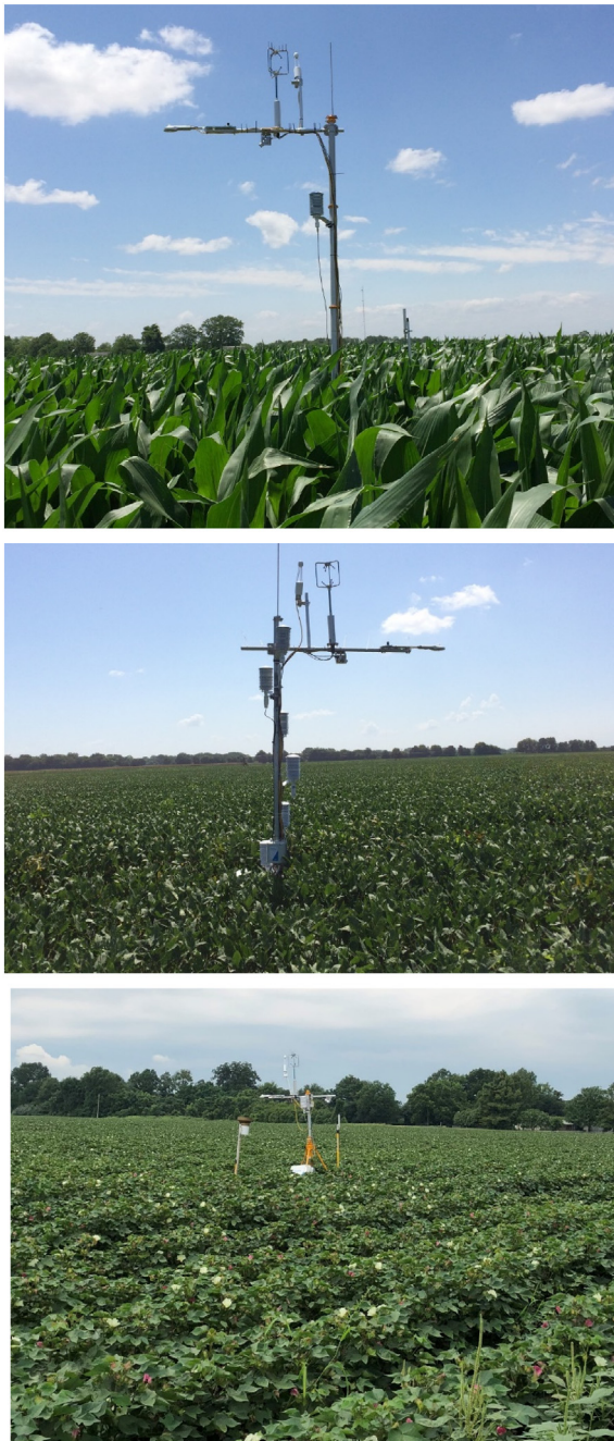
Fig. 1. The eddy covariance system installed in corn (top panel), soybean (middle panel), and cotton (bottom panel) fields for measuring net ecosystem exchange of CO 2 and water.
